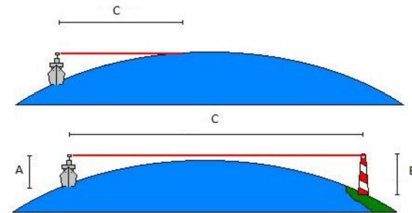
Figure 19.1: Determining Radar range.
