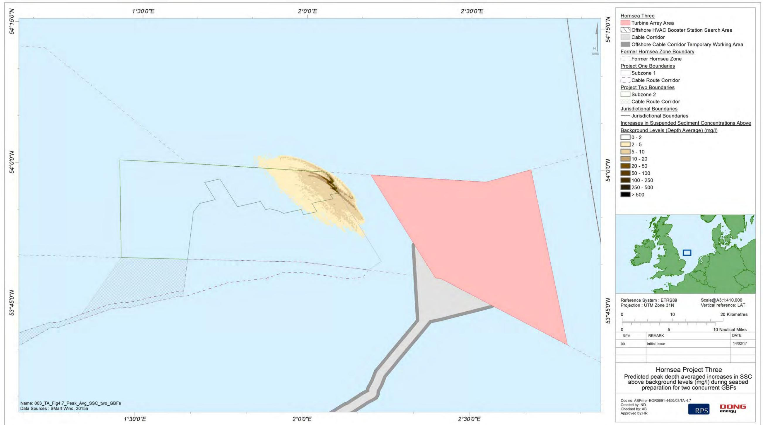
Figure 4.7: Predicted peak depth averaged increases in SSC above background levels (mg/l) during seabed preparation for two concurrent gravity base foundations (reproduced from SMart Wind, 2015a).
