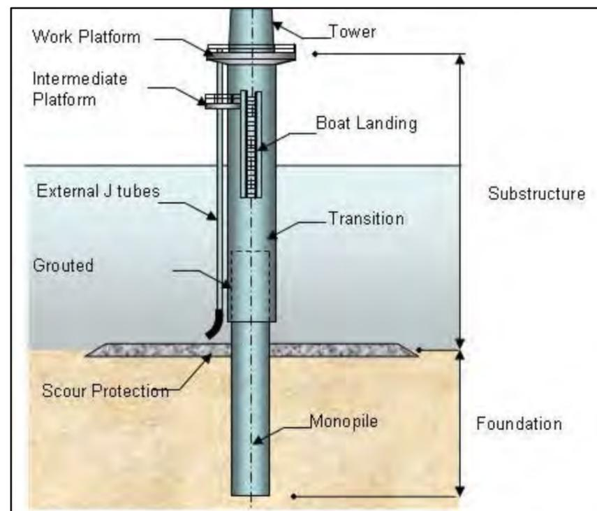
Figure B.1: Outline design of a typical steel monopile foundation (with scour protection) (reproduced from SMart Wind, 2015d).
