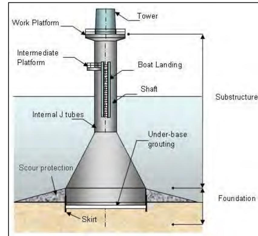
Figure B.3: Outline design of a gravity base foundation (reproduced from SMart Wind, 2015d).
