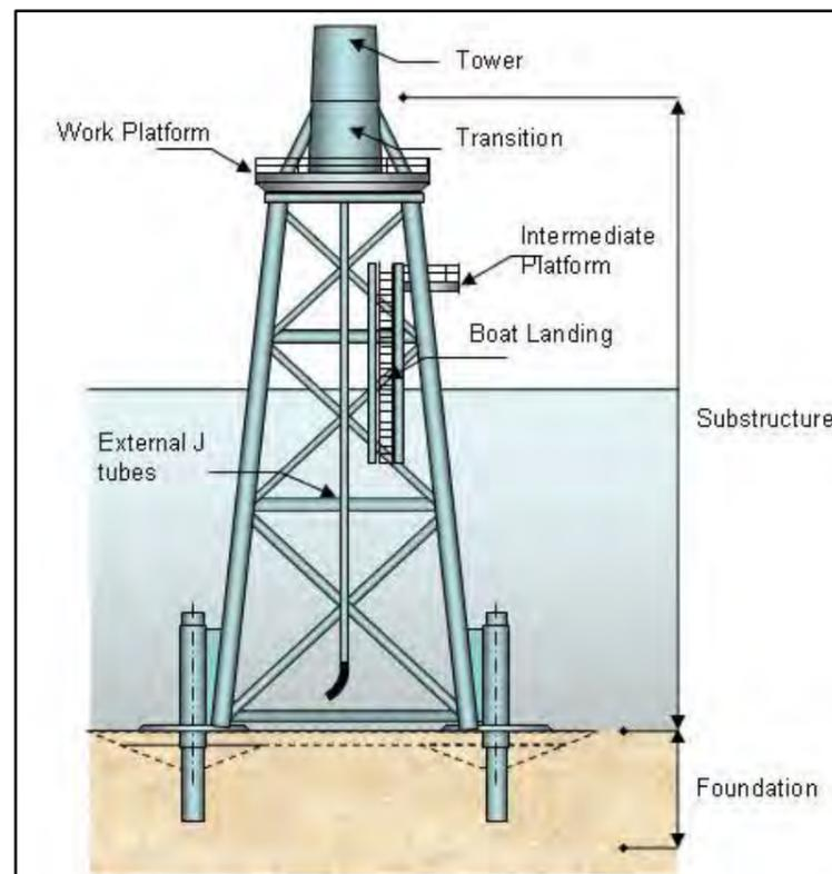
Figure B.2: Outline design of a typical jacket foundation (reproduced from SMart Wind, 2015d).
