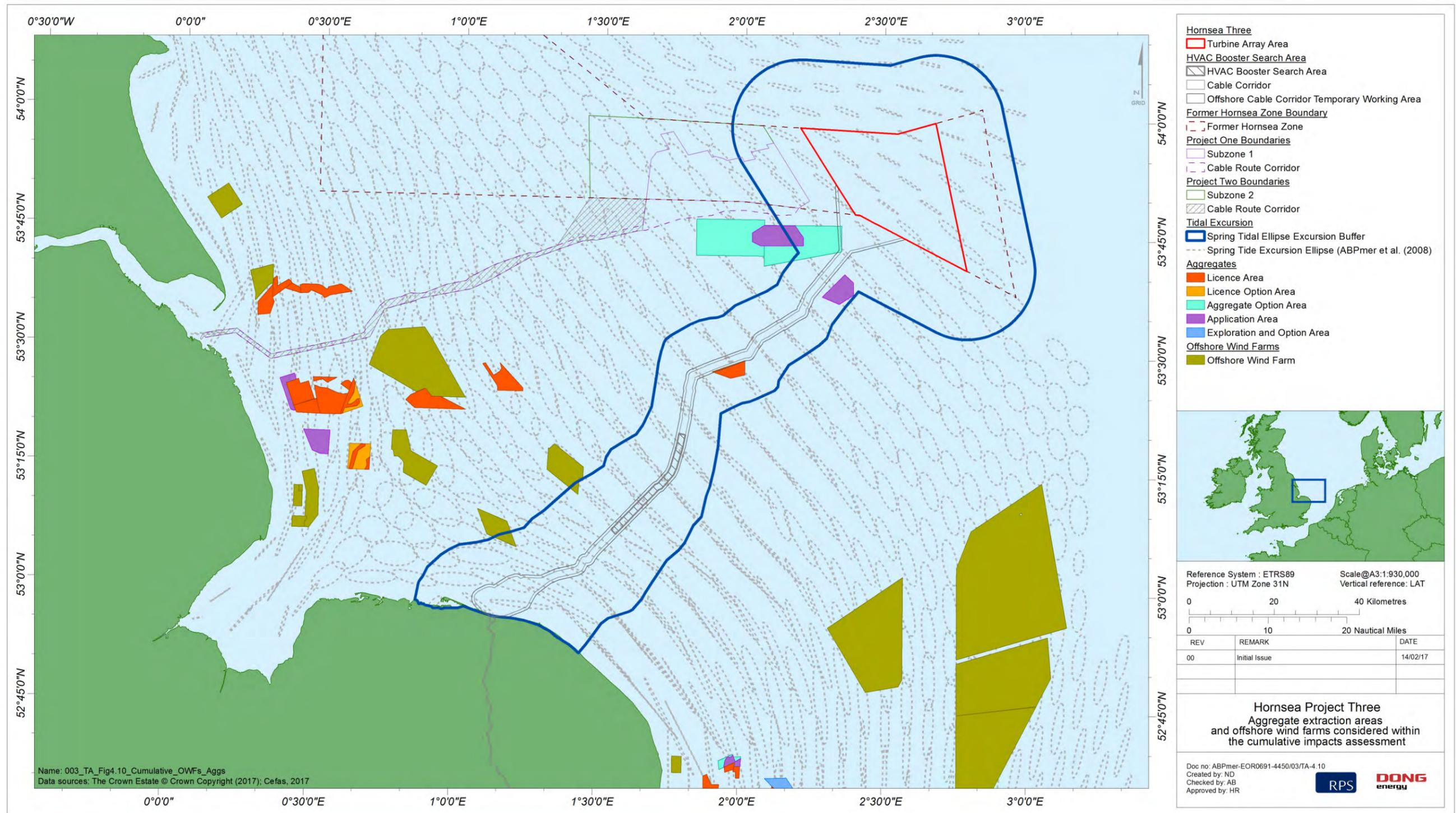
Figure 4.10: Aggregate extraction areas and offshore wind farms considered within the cumulative impacts assessment.
