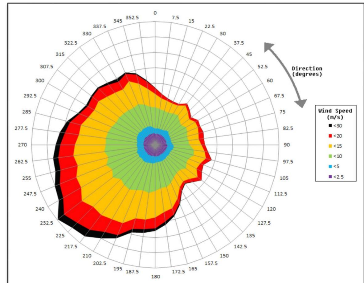
Figure 7.6: Wind speed and direction frequency distribution for 2002 to 2012.
