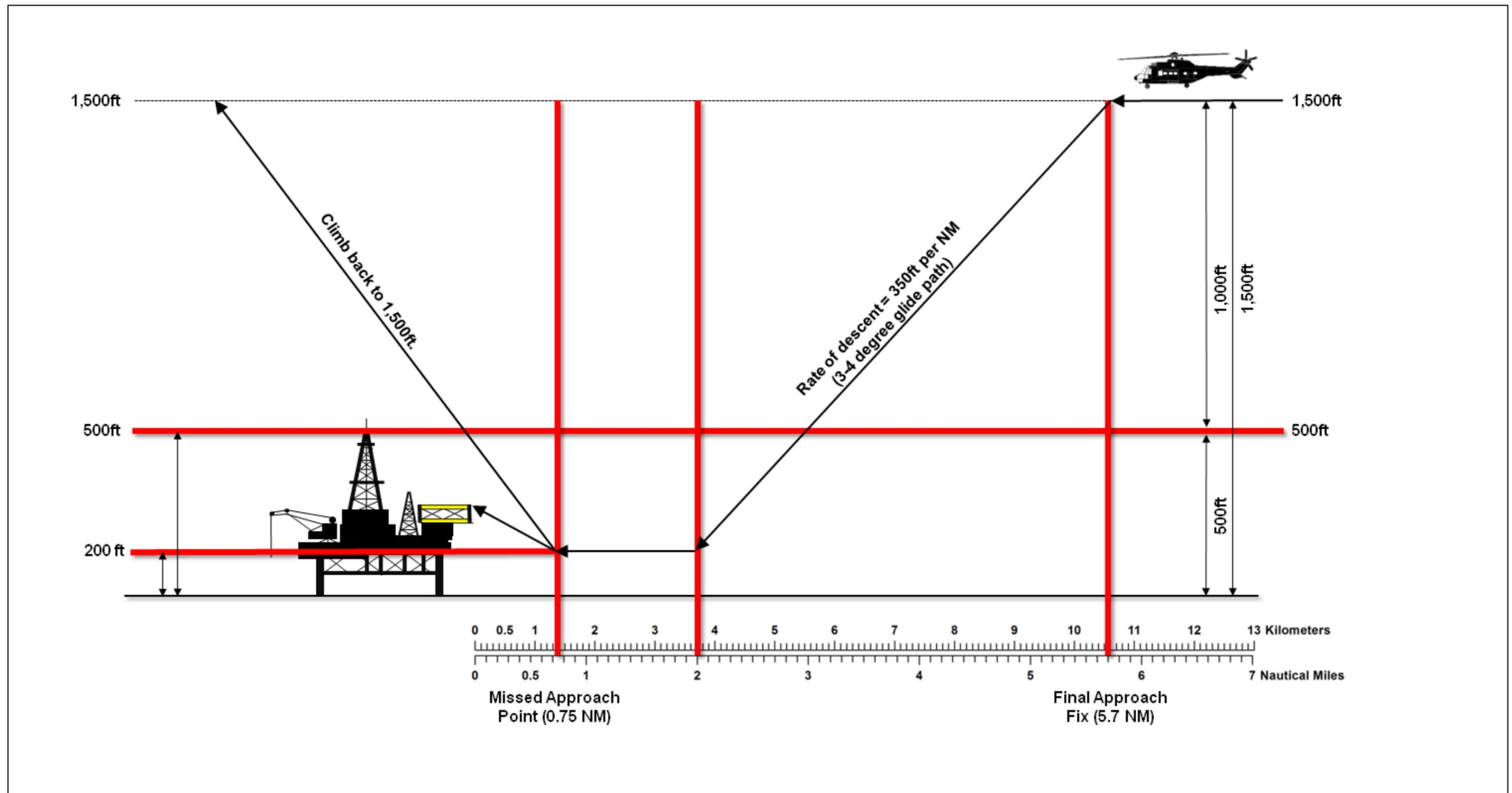
Figure 7.4: Indicative instrument approach procedure without turbines present.
