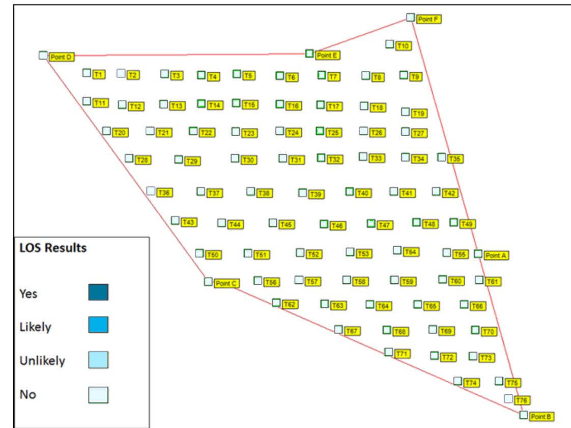
Figure 5.1: LOS Results from NATS Claxby PSR at a turbine tip height of 325 m.
