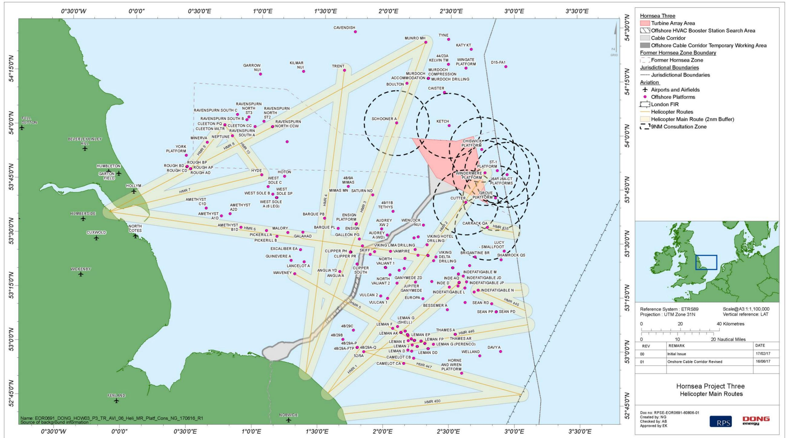
Figure 7.1: The HMR structure and 9 nm consultation zones which intersect with the Hornsea Three array area.
