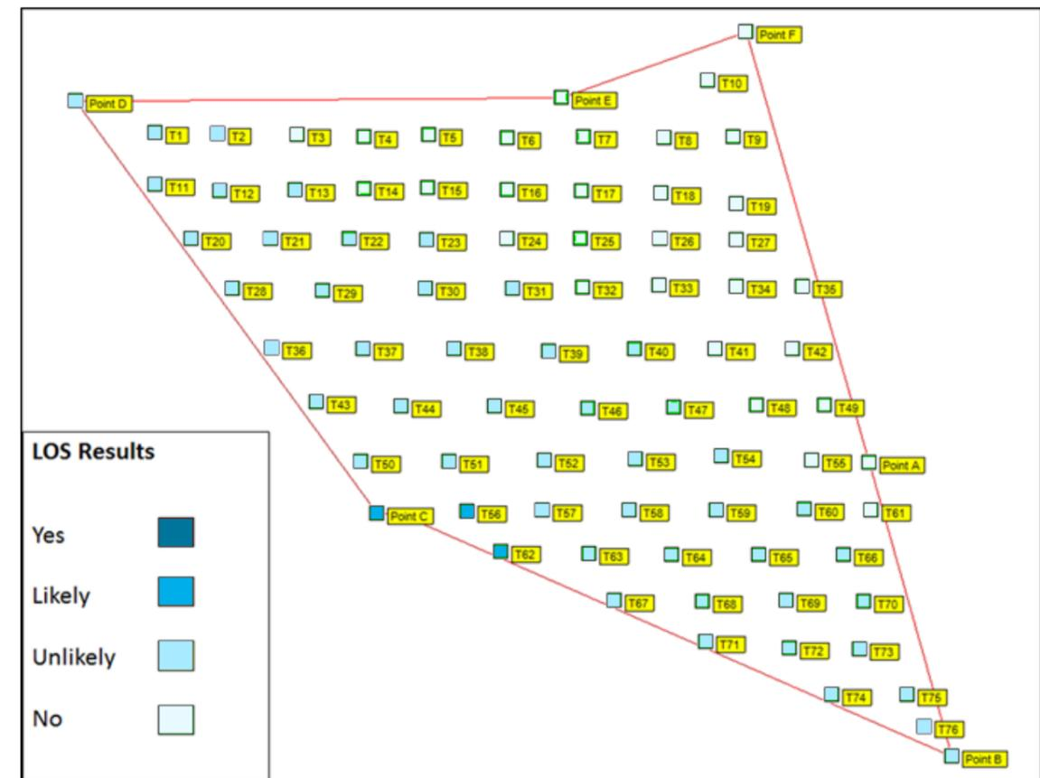
Figure 6.2: LOS results from MOD Trimmingham ADR at a turbine tip height of 325 m.
