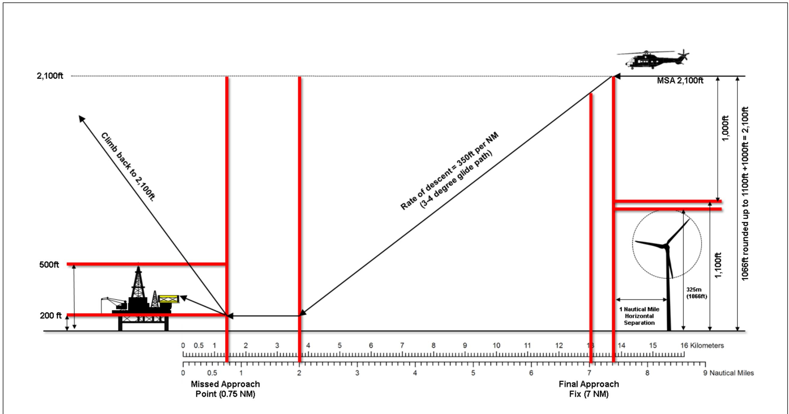
Figure 7.5: Indicative instrument approach procedure with turbines present.
