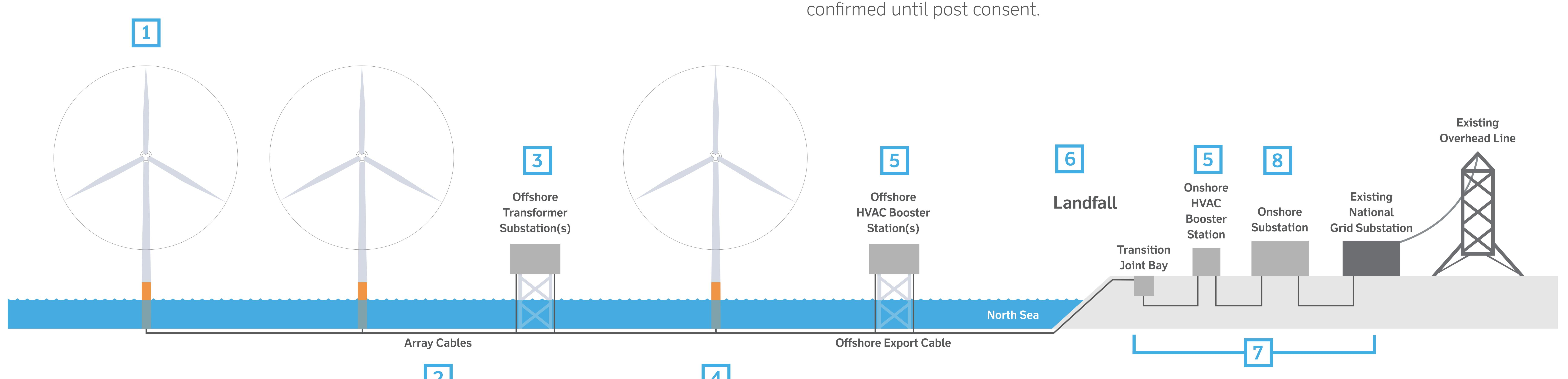
2. A new network of subsea array cables will connect the wind turbines, offshore substation(s), offshore converter stations and offshore accommodation platforms.
