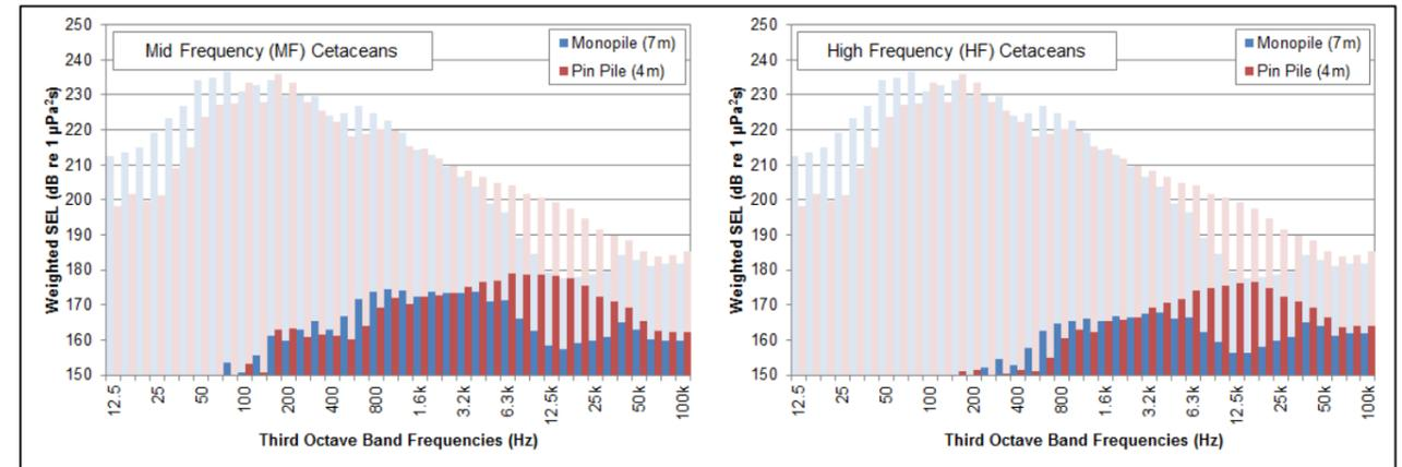
Figure 5.18: Filtered noise inputs for monopiles and pin piles using the MF cetacean and HF cetacean filters from NMFS (2016). The greyed bars show the unweighted third octave levels.
