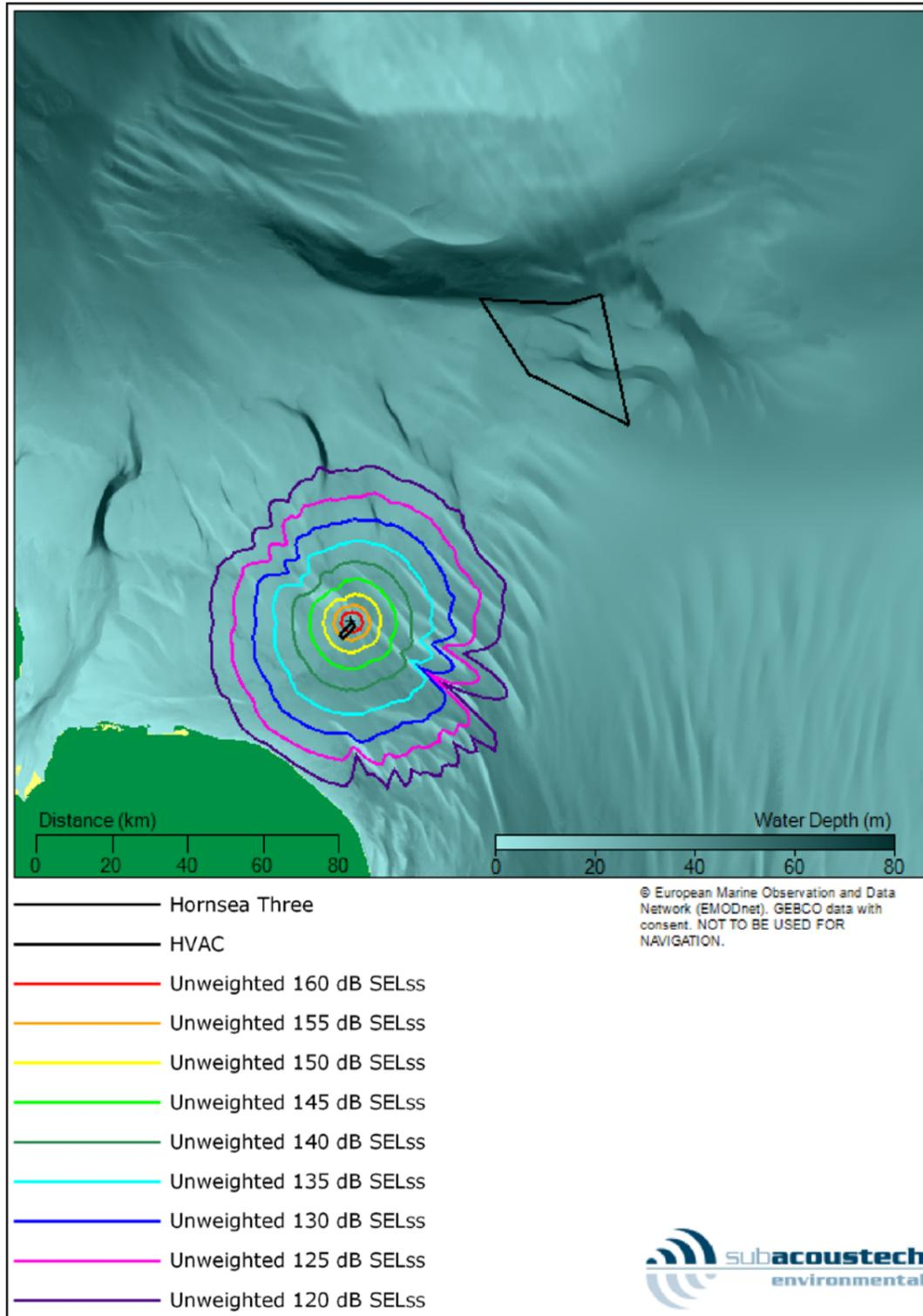
Figure 5.6: Contour plot showing the modelled unweighted SEL<sub>ss</sub> noise levels at the HVAC N location for installing a monopile with a maximum blow energy of 5000 kJ.
