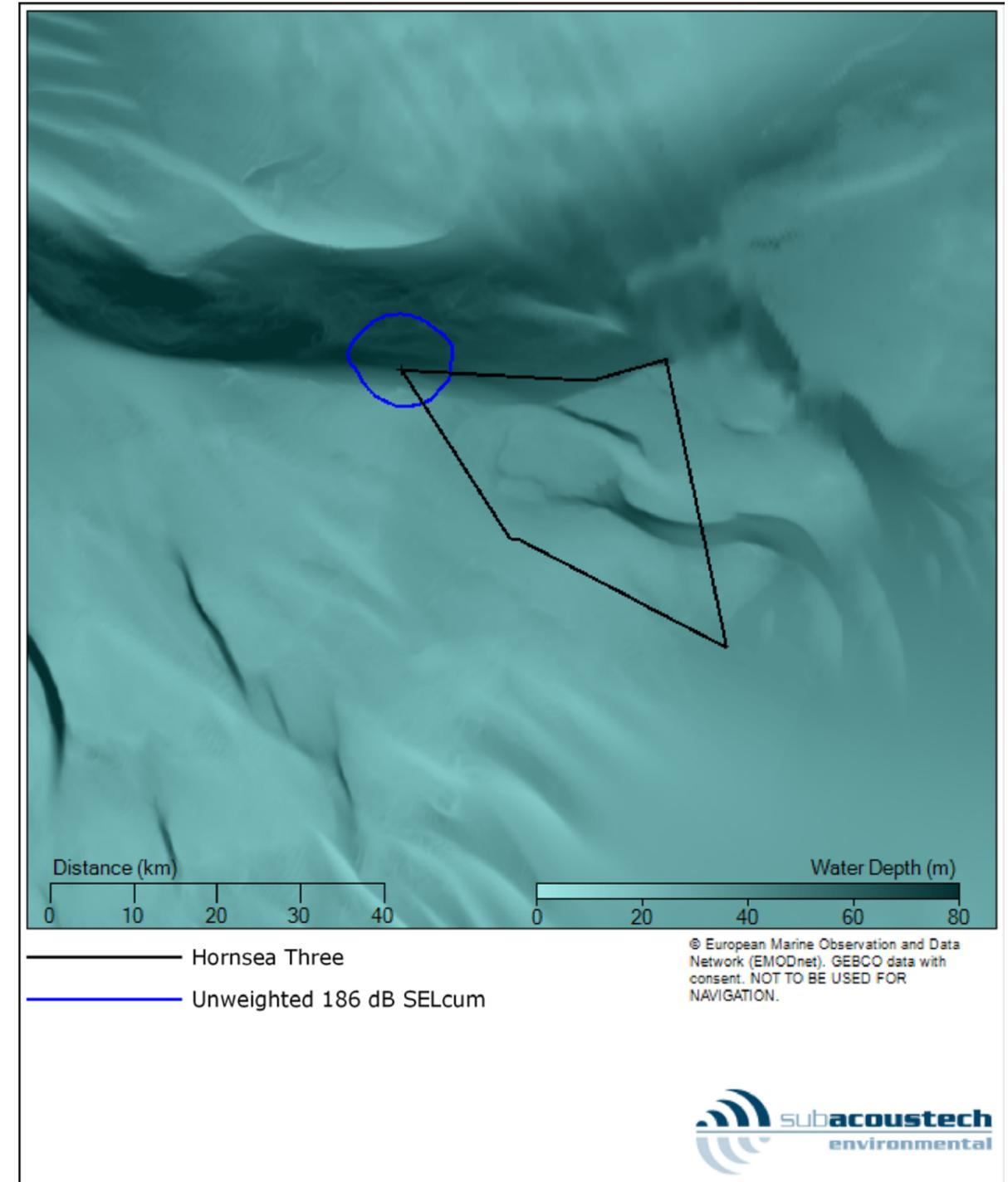
Figure 5.20: Contour plot showing the unweighted SEL<sub>cum</sub> TTS impact ranges (Popper et al. 2014) for fleeing fish at the NW location for installing a pin pile with a maximum blow energy of 2500 kJ.
