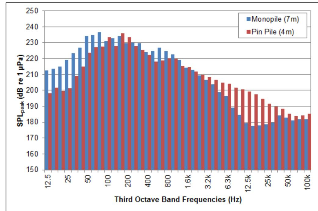
Figure 5.2: Third octave source level frequency spectra for the NW location, maximum blow energy.
