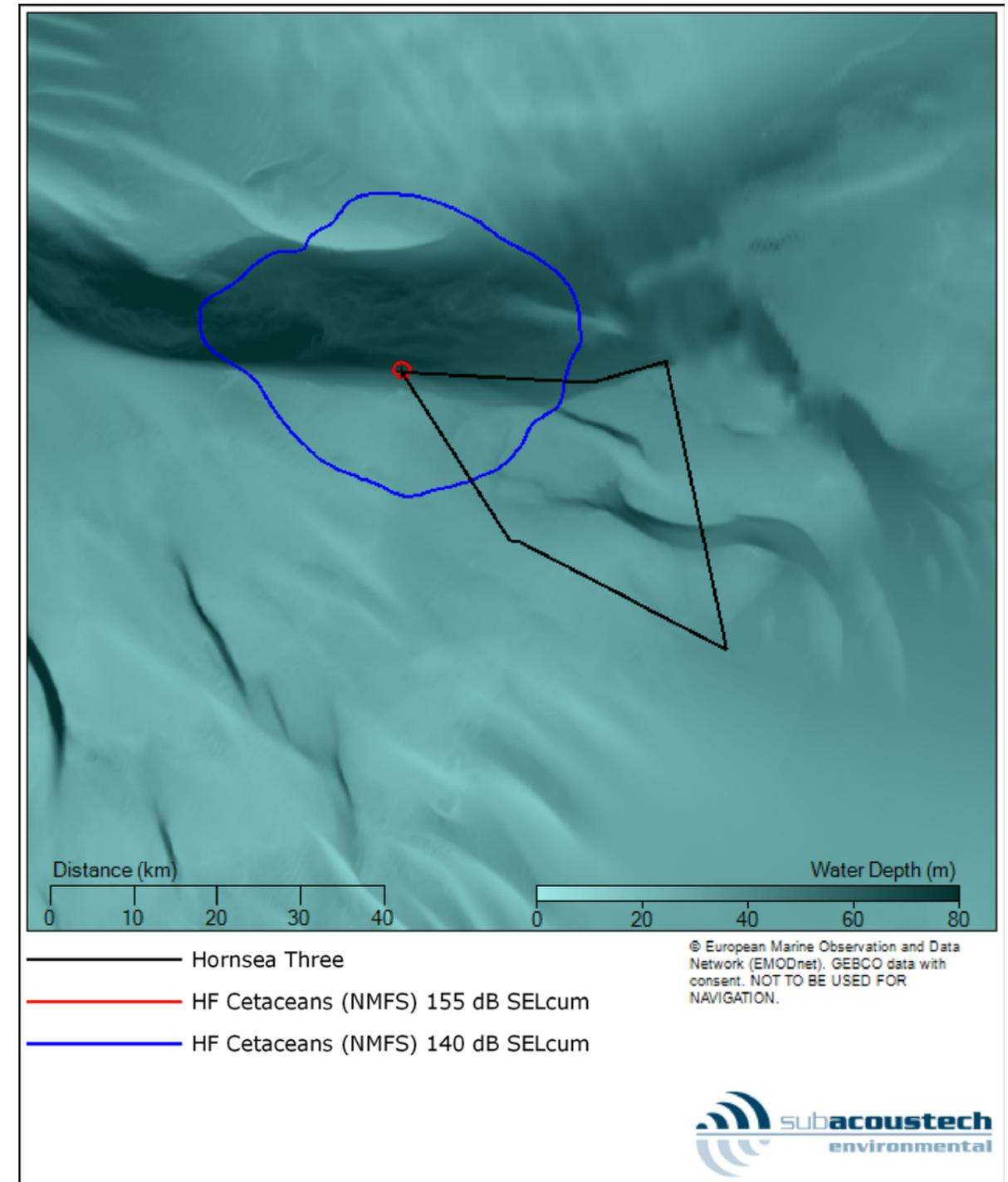
Figure 5.15: Contour plot showing the modelled PTS and TTS impact ranges (NMFS, 2016) for fleeing high frequency (HF) cetaceans at the NW location for installing a pin pile with a maximum blow energy of 2500 kJ.
