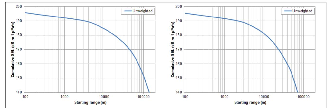
Figure 5.23: Total received cumulative SEL for species of fish (Popper *et al.* (2014) unweighted criteria) when fleeing from impact piling noise at NW location for a monopile installed with a maximum hammer energy of 3500 kJ (Left plot = WNW transect (290°), Right plot = SSW transect (190°)).
