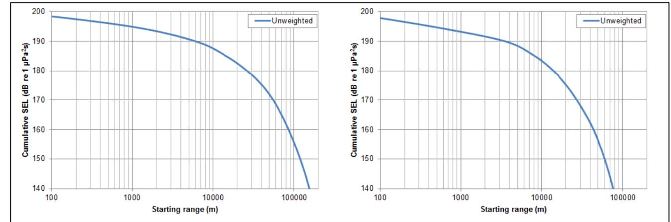
Figure 5.22: Total received cumulative SEL for species of fish (Popper *et al.* (2014) unweighted criteria) when fleeing from impact piling noise at NW location for a monopile installed with a maximum hammer energy of 5,000 kJ (Left plot = WNW transect (290°), Right plot = SSW transect (190°)).
