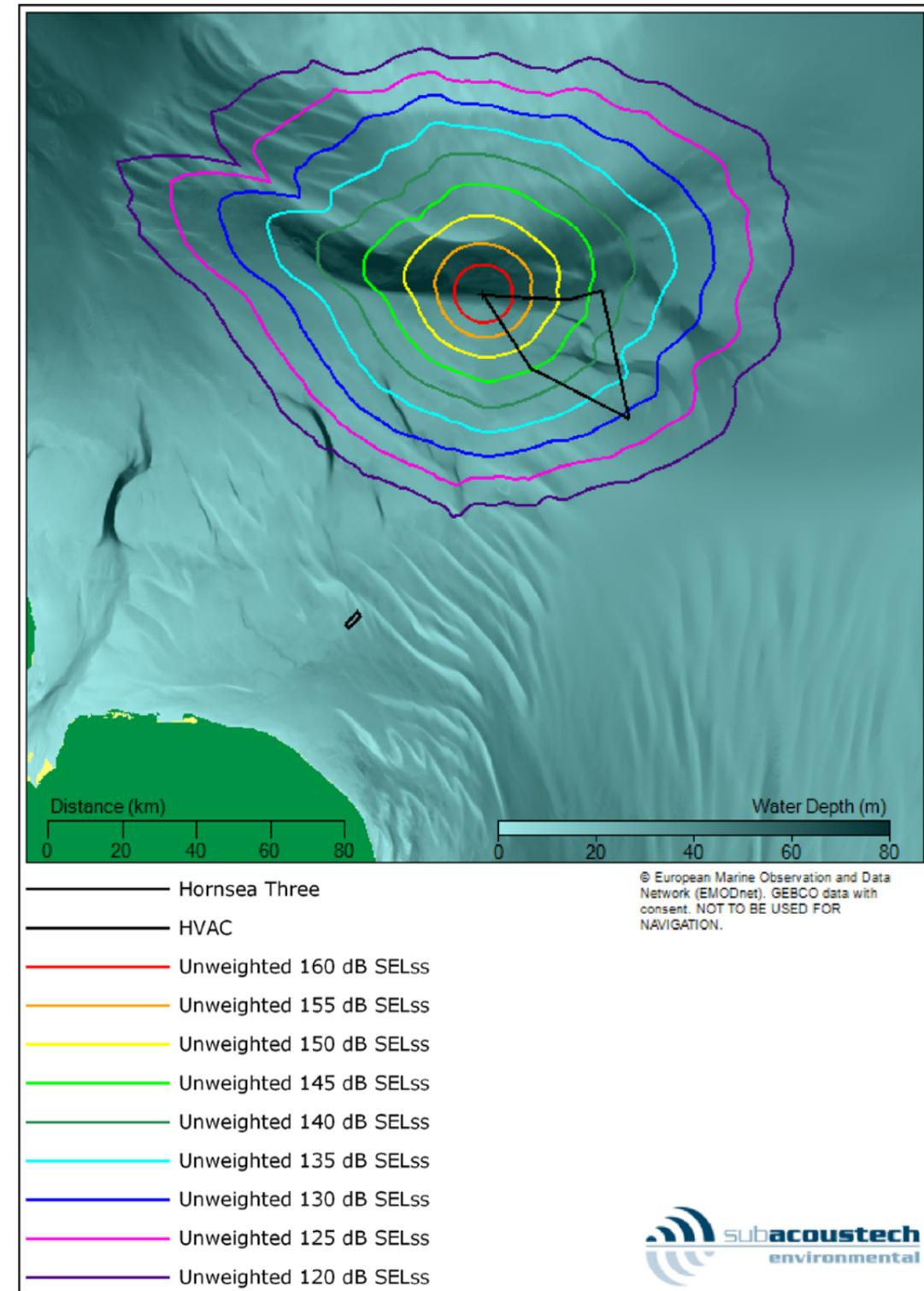
Figure 5.3: Contour plot showing the modelled unweighted SEL<sub>ss</sub> noise levels at the NW location for installing a monopile with a maximum blow energy of 5000 kJ.
