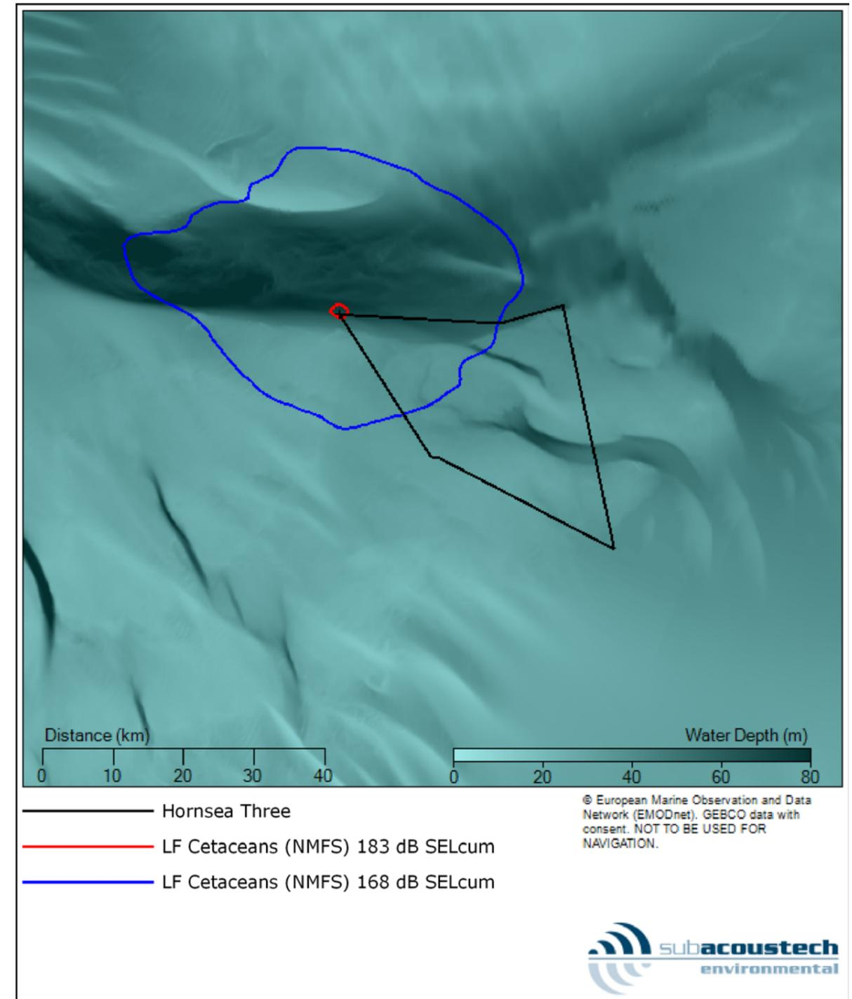
Figure 5.11: Contour plot showing the modelled PTS and TTS impact ranges (NMFS, 2016) for fleeing low frequency (LF) cetaceans at the NW location for installing a monopile with a maximum blow energy of 5000 kJ.
