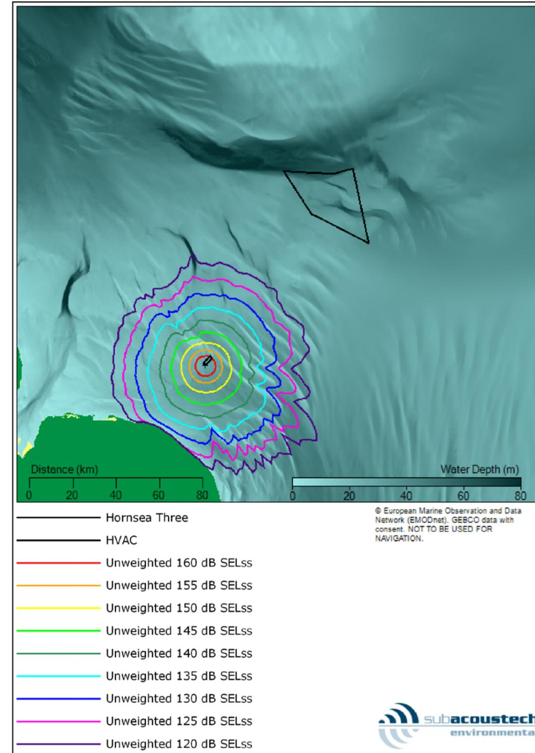
Figure 5.7: Contour plot showing the modelled unweighted SEL<sub>ss</sub> noise levels at the HVAC S location for installing a monopile with a maximum blow energy of 5000 kJ.
