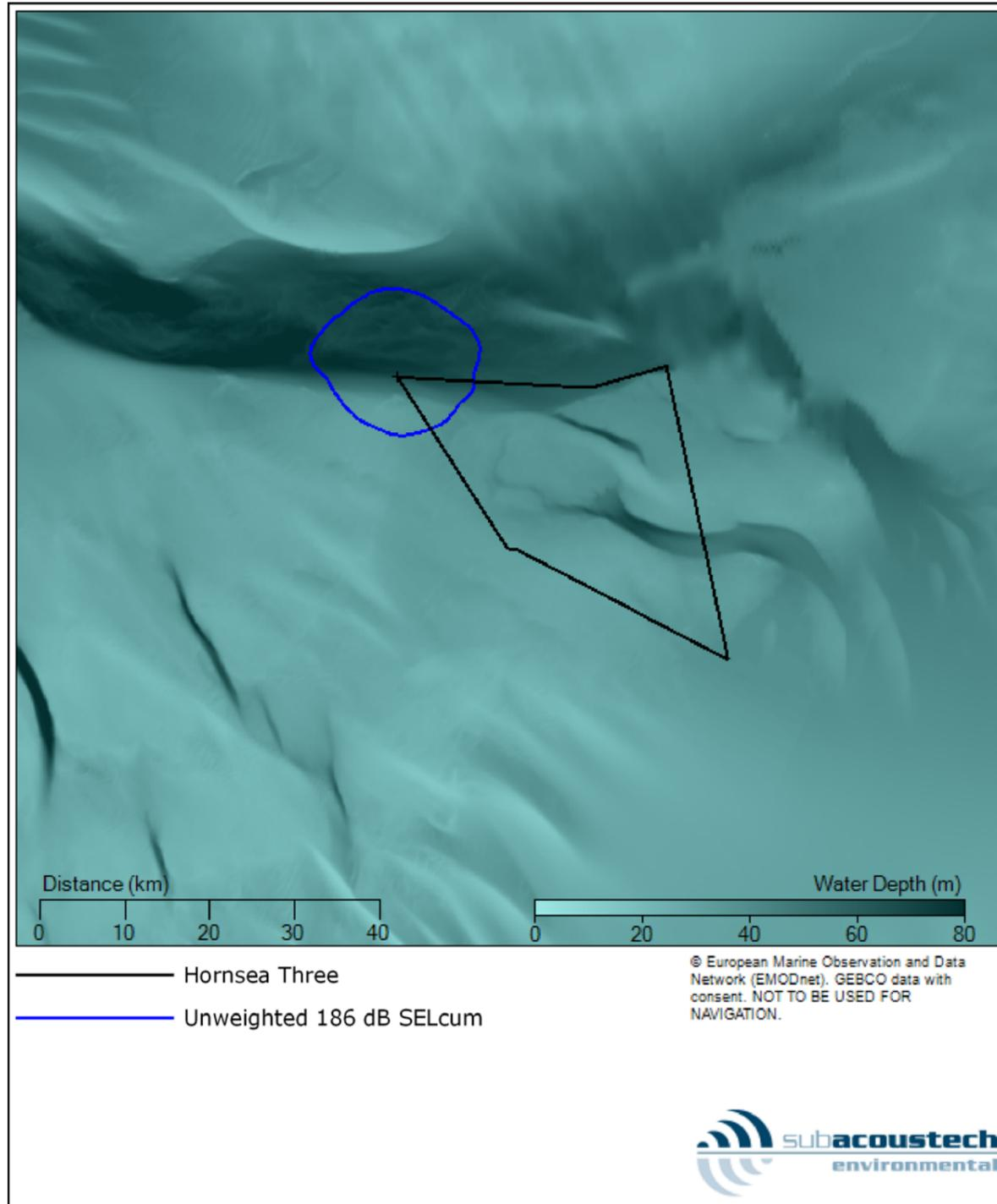
Figure 5.19: Contour plot showing the unweighted SEL<sub>cum</sub> TTS impact ranges (Popper et al. 2014) for fleeing fish at the NW location for installing a monopile with a maximum blow energy of 5000 kJ.
