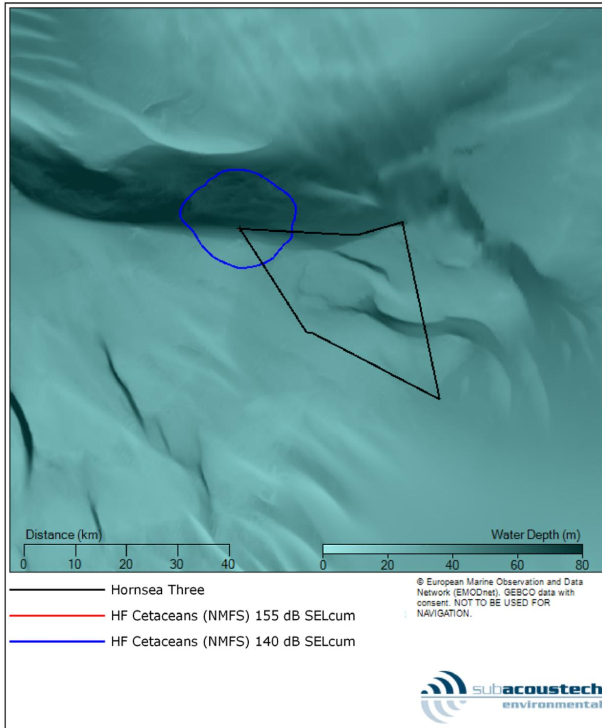
Figure 5.12: Contour plot showing the modelled PTS and TTS impact ranges (NMFS, 2016) for fleeing high frequency (HF) cetaceans at the NW location for installing a monopile with a maximum blow energy of 5000 kJ. Note the 155 dB contour is too small to be visible at this scale.
