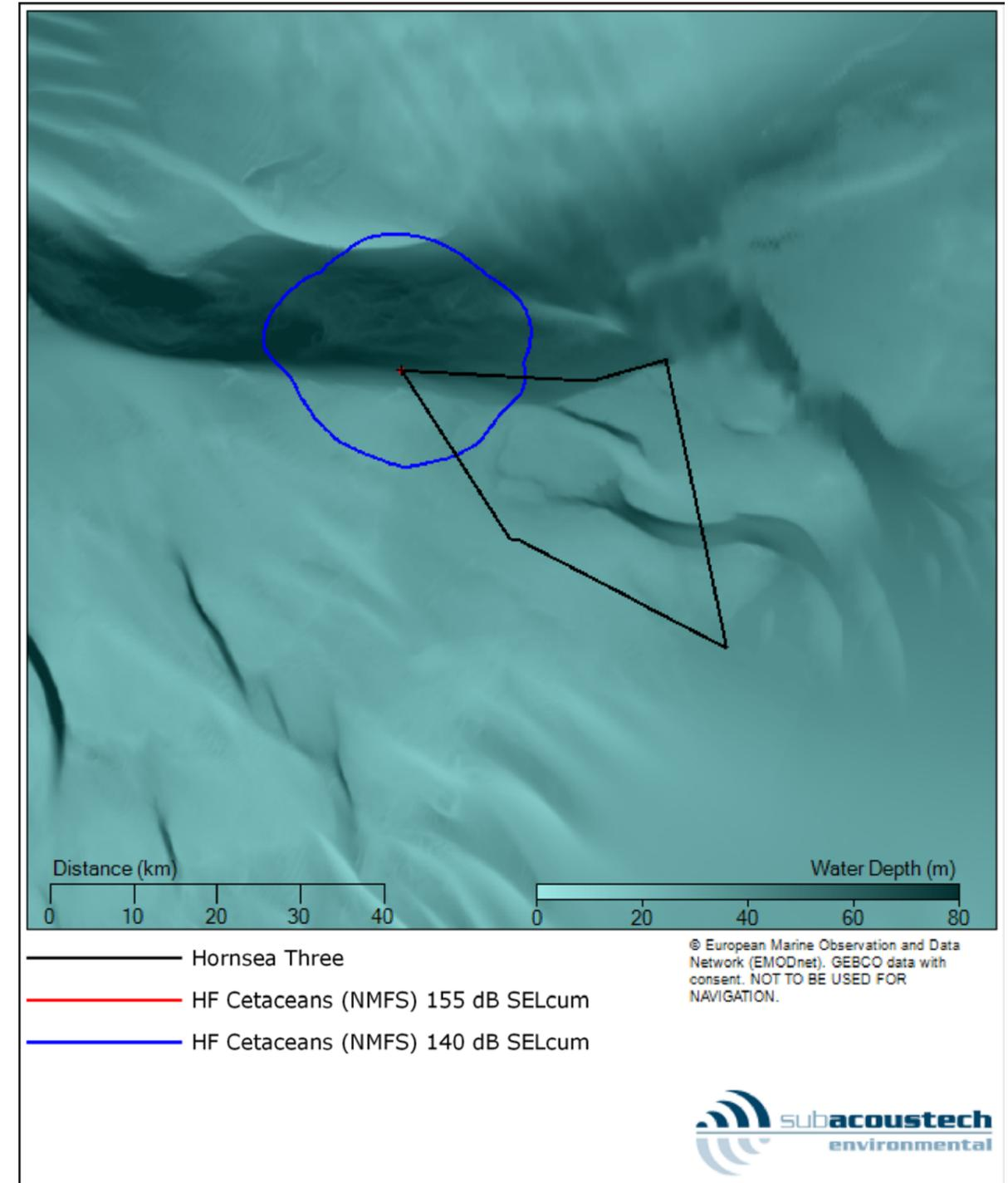
Figure 5.17: Contour plot showing the modelled PTS and TTS impact ranges (NMFS, 2016) for fleeing high frequency (HF) cetaceans at the NW location for installing a pin pile with a Most Likely maximum blow energy of 1750 kJ.
