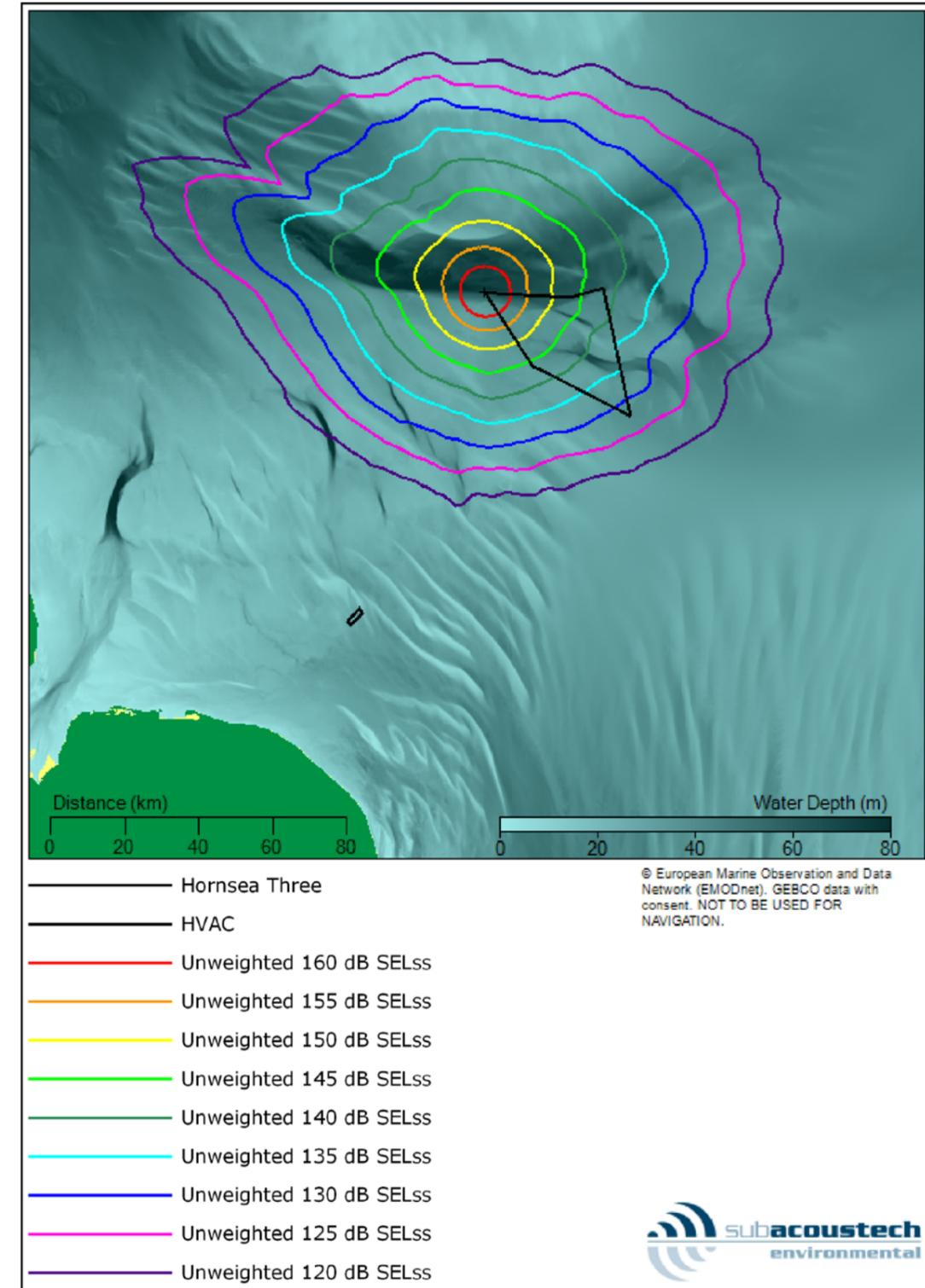
Figure 5.9: Contour plot showing the modelled unweighted SEL<sub>ss</sub> noise levels at the NW location for installing a monopile with a maximum blow energy of 3500 kJ.
