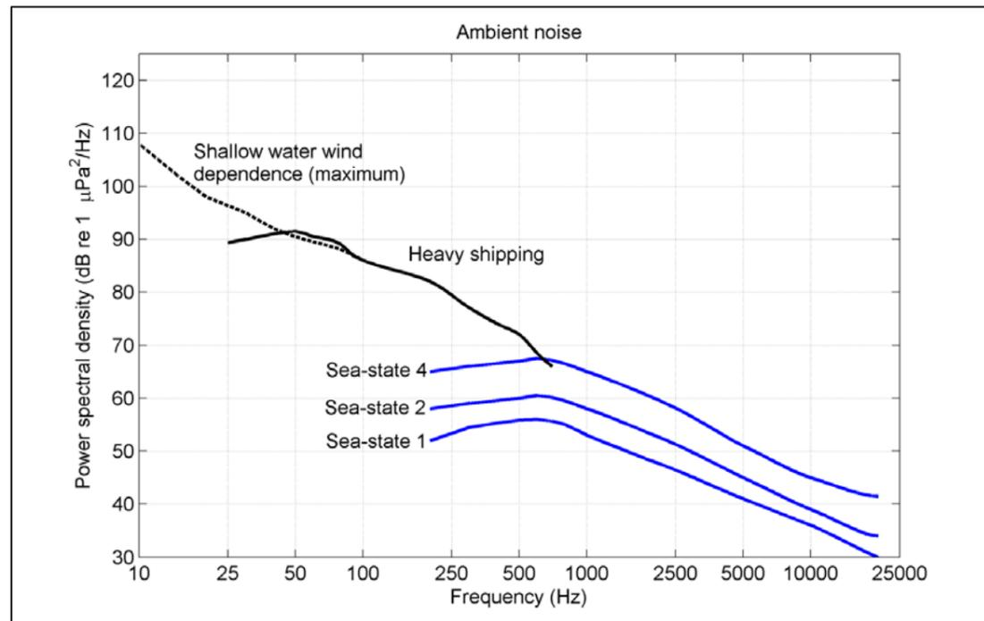
Figure 4.1: Ambient underwater noise as shown in Wenz (1962) showing frequency dependency from different noise sources.
