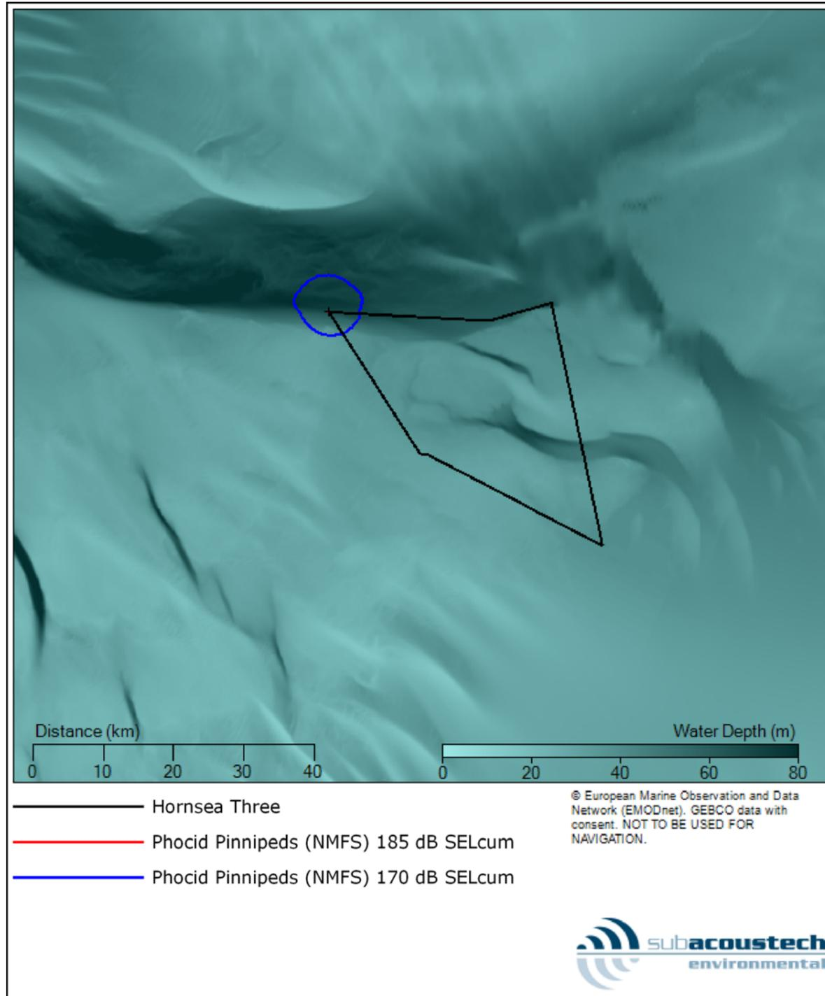
Figure 5.16: Contour plot showing the modelled PTS and TTS impact ranges (NMFS, 2016) for fleeing phocid pinnipeds (PW) at the NW location for installing a pin pile with a maximum blow energy of 2500 kJ. Note the 185 dB contour is too small to be visible at this scale.
