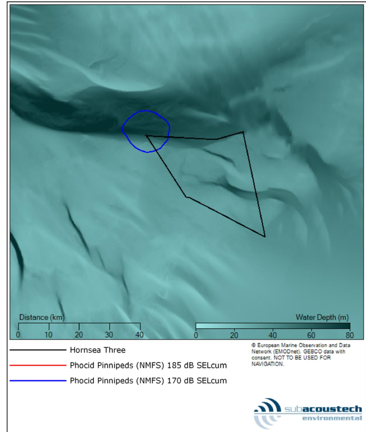
Figure 5.13: Contour plot showing the modelled PTS and TTS impact ranges (NMFS, 2016) for fleeing phocid pinnipeds (PW) at the NW location for installing a monopile with a maximum blow energy of 5000 kJ. Note the 185 dB contour is too small to be visible at this scale.
