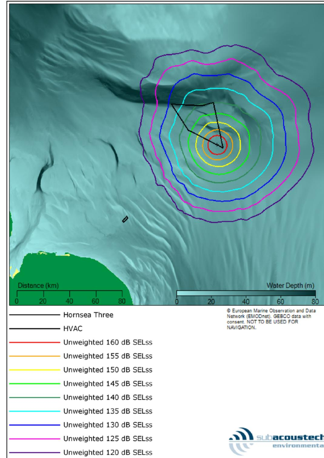
Figure 5.4: Contour plot showing the modelled unweighted SEL<sub>ss</sub> noise levels at the NE location for installing a monopile with a maximum blow energy of 5000 kJ.
