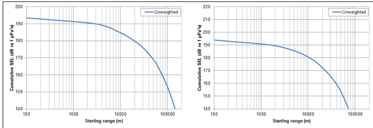
Figure 5.24: Total received cumulative SEL for species of fish (Popper *et al.* (2014) unweighted criteria) when fleeing from impact piling noise at NW location for a pin pile installed with a maximum hammer energy of 2,500 kJ (Left plot = WNW transect (290°), Right plot = SSW transect (190°)).
